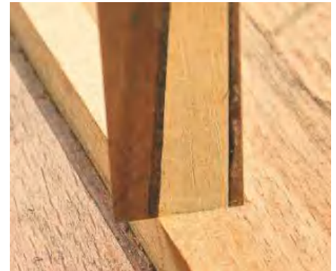
▲ Pic.7 Here the blade is vertical but the edge is out of square
